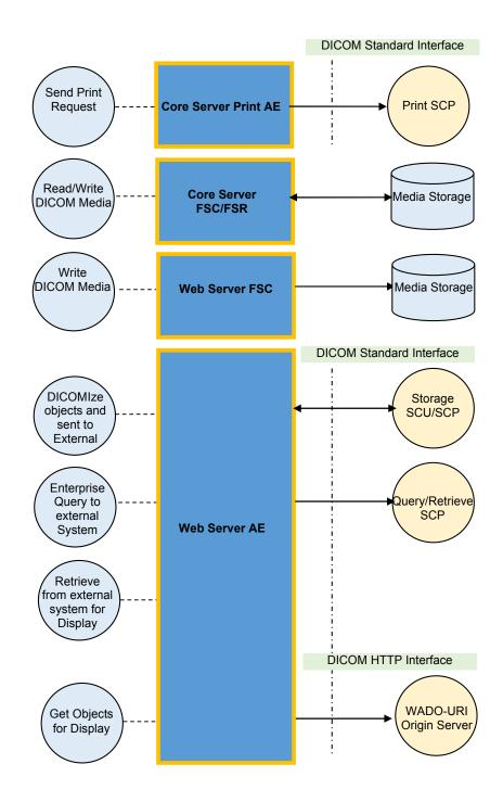
Figure 4-2 Enterprise Imaging Application Data Flow Diagram Part 2
