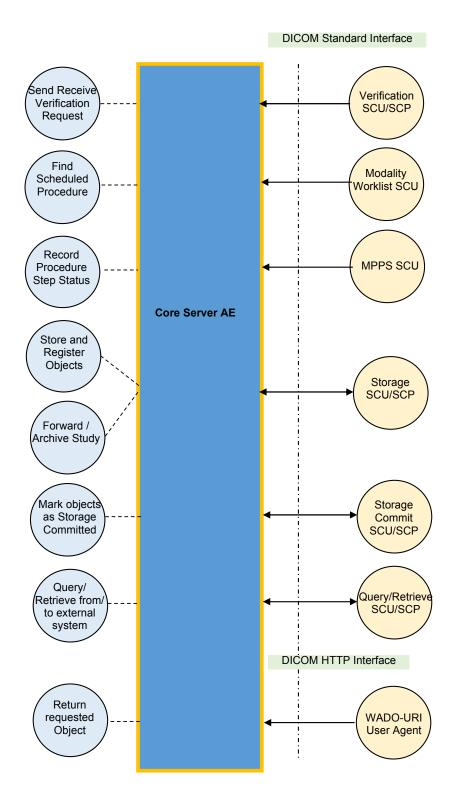
Figure 4-1 Enterprise Imaging Application Data Flow Diagram part 1
