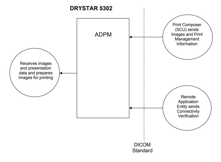
Figure 2.1-1: Functional Overview – Application Data Flow
