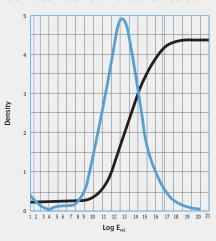
Machine processing MAMORAY HT-300 with RP processing cycle. Agfa Mammography Chemistry. X-Rite Sensitometer.
